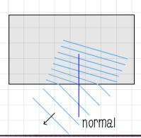
When waves leave glass, they speed up increasing the wavelength.
