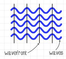
The wavefront is an line that connects all the same points in a group of waves. In the diagram on the left, the wavefronts have been drawn by connecting the peaks of each wave.
