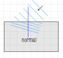
When the first part of the wavefront move into the glass, the wavefronts slows down. Note how the wavefronts become closer (shorter wavelength). This causes the wave to change direction towards the normal.
