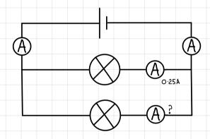
Calculate the current in the second branch of the parallel circuit
