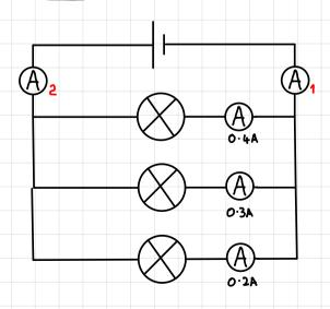
Calculate the current at A1 and A2 in the parallel circuit
