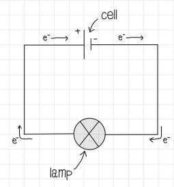
The electric current flows from the negative end of the cell to the positive end.
