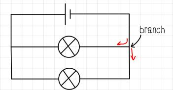
A parallel circuit contains branches. The current is divided through both of the branches
