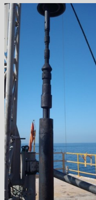
Lock + straddle fished from well
