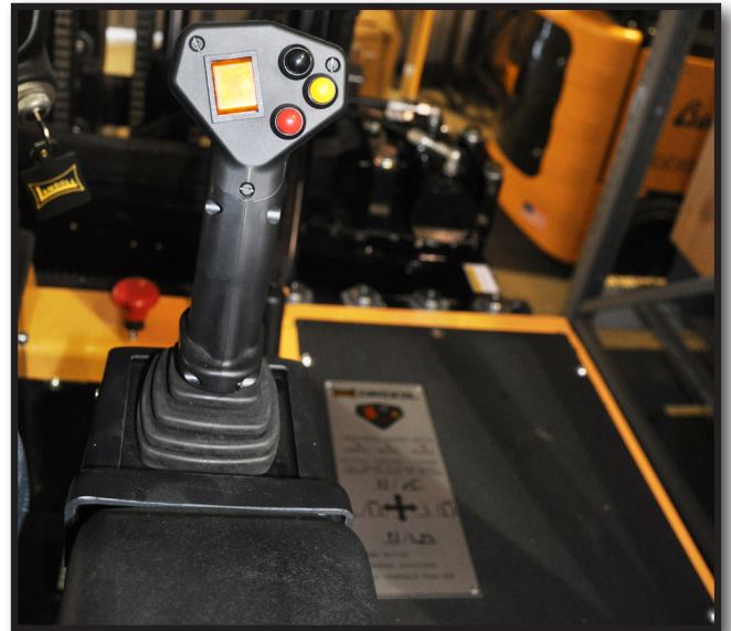
Single Joystick Controls for All Hydraulic Functions, Directional Control and Horn
