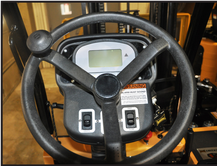
Dash Display with Full Diagnostics, Hour Meter and Battery Discharge Indicator
