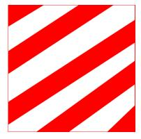
Equipment Free Zones are red hatched areas. Equipment must not be staged or stored within these areas. Aerobridges are marked with Equipment Free Zones
