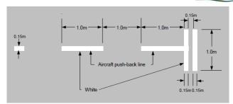
Pushback lines are only provided where the pushback differs from the lead-in line. The Tug Operator must disconnect at the relevant Tug Disconnect Point (TDP) for the bay in which the pushback commenced.
