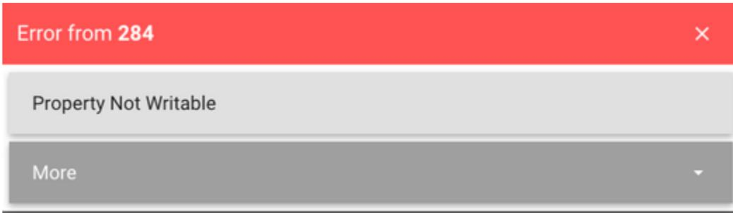
The board sent back an error response to the "SET". This make sense because for an input pin, you can only read the value. You cannot set it.
