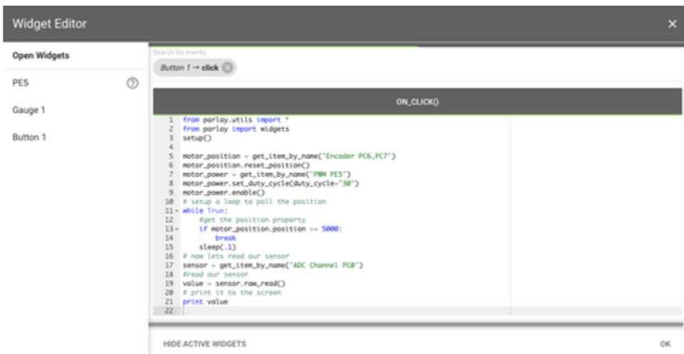
Note that if we run this, we will be in the loop forever because we do not have a motor with encoder attached. However, should you run it, you can stop it with the button's menu Stop Script, as shown below:
