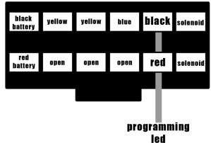
INSTALLING THE PROGRAMMING LED LIGHT Since the Freestyle does not have an LED indicator you will need to install the one that we included with your newly flashed board. We have shipped a small RED LED with BLACK and RED wires attached. (Black and White wire shown in the image above.)
