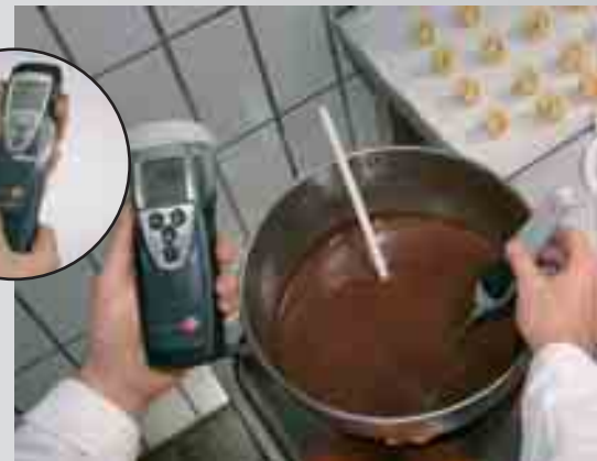
Checks the exact temperature of freshly melted chocolate, no annoying cable thanks to the use of the radio probe
