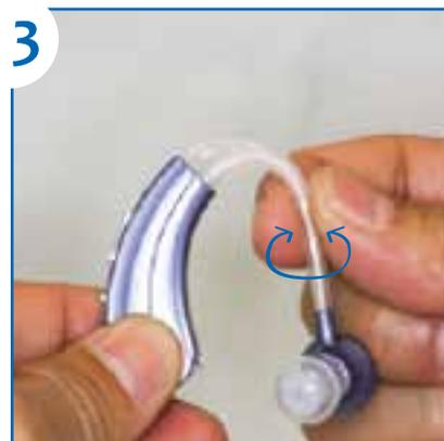
3 The Amplifier Tube can be turned left or right to fit either Ear.
