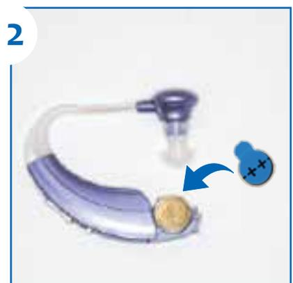
2 Remove Sticker from Battery, open the Battery Gate and install Battery with (+) positive sign facing up.
