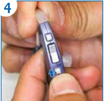
4 Move Power Switch to the "ON" (up) position.
