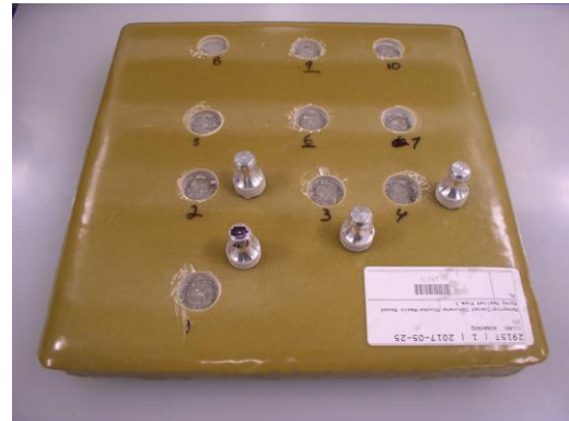
Figure 13 Concrete Plate after Test
