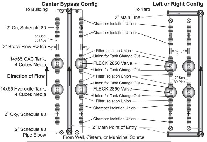
2" INLET, BYPASS IS STRAIGHT THROUGH
