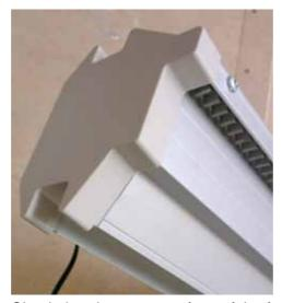
Check that the upper surface of the footrest is no further than 6  $\frac{1}{2}$ " above bottom and top boarding points. Adjust end stop / charge points to suit.
