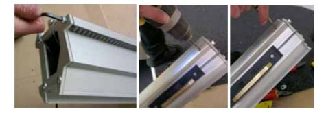
Slacken off rack tension bolt but leave in place. Fit plastic end cap.
