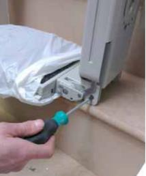
Attach Chassis Leg to Drive Unit ensuring all cables pass through central hole correctly. Fit washers and nuts, tightening one to temparily hold Chassis Leg in position.
