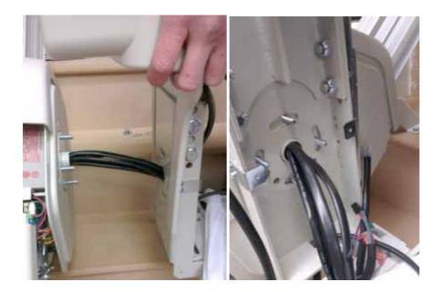
Connect Powered Swivel Motor Ioom (Red & Black), connect Footrest Ioom (Yellow & Brown).
