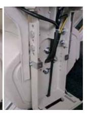
Fit Seat using 4 x 5mm Allen bolts. Using a torque wrench, Tighten to 20 Nm. Connect Chair and Display Looms. Lift manual swivel levers and turn chair, make sure it locks securly at either end if travel and thet the swivel interlock switch operates correctly.
