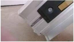
If charger is to be located at bottom of the stairs drill 12.5mm hole in underside of rail, fit cable gland and pass charge wire through. Connect Black core with white trace to connector block. Crimp ring connector on to Black charger core and 0v core through rail. Loosen end cap and clamp Crimp ring connector between end cap and rail. Tighten cable gland. This procedure can also apply to the top if the charger is to be located there.
