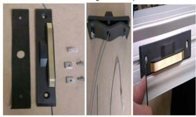
The charge/end stop assembly determines the height of the stairlift finishing postion at the bottom of the stairs. The assembly must be at least 2 ½" from the end of the rail. Note: Be careful not to allow the charging wire to be trapped under the screw when tightening the charging point in place Fit rail end cap.
