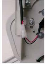
Connect Swivel Limit Ioom (Purple & White) to swivel limit switches as shown in the picture below, White pair always connected to the right hand switch, COM and N.O, purple pair to left hand switch, COM and N.O. Finally pass chair and display loom through centre of swivel boss.
