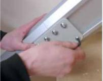
Run supplied 2 core cable down the inside of the rail and connect +ve core to grey charge strip cable using connector block.
