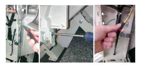
Remove plastic footrest cover, remove footrest limit loom, slacken off grub screw.
