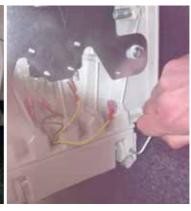
Tap mounting bar through bracket and remove footrest assembly, pull loom out of footrest 1 connector at a time, remove 3 bolts and repostion bracket. Replace bolts and feed loom back through hole 1 connector at a time. Reattach to chassis leg by knocking mounting bar back through bracket – be careful not to damage footrest limit loom. Tighten grub screw and reattach lever link bracket with 2 screws. Rehook leverlink footrest spring.
