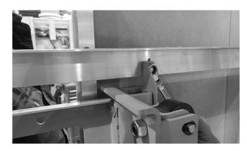
▲ ACCESS EACH HEX BOLT FROM THE T1 INNER PANEL. ENSURE EACH HEX BOLT ON EACH SIDE IS FIRMLY TIGHTENED.
