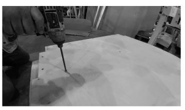
▲ Ensure the 6 Flat Head Machine Screws are firmly fastened.
