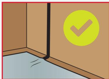
Position the power cord so it sits securely into the corner of the base and side wall of the IBC without bridging or creating tension.
