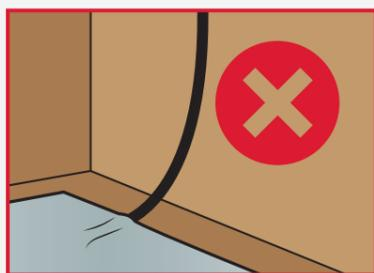
Make sure no excess power cord comes into contact with any heater surface.
