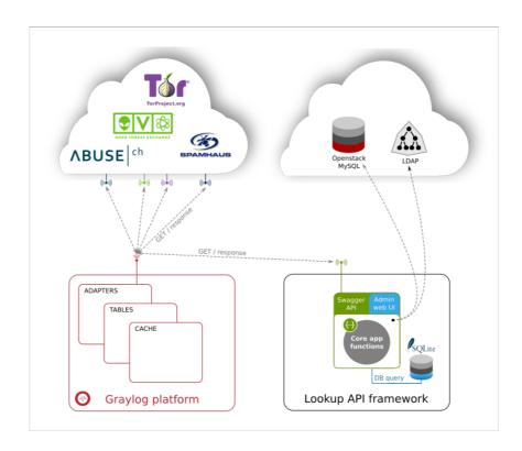
Lookup API framework aggregates multiple data sources, internal as well as external. Information inside are collected and re-generated on a scheduled basis.
