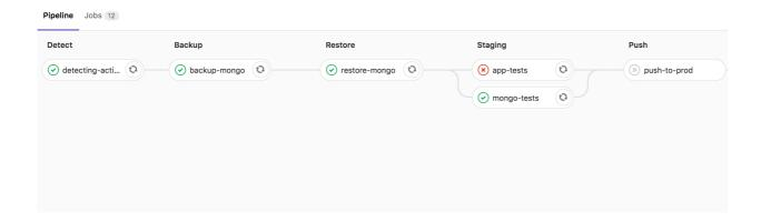
Remaining part of the pipeline did not run due to failed staging test. I.e. issues have been correctly caught in STAGE environment and not propagated to PROD:
