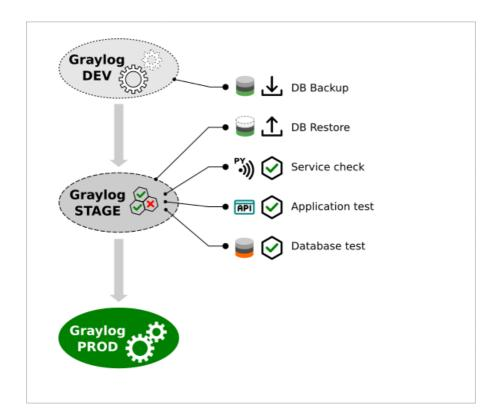
Implemented CICD helps also to keep up with Graylog release cycles in an easy way to avoid surprises when upgrading across multiple versions. Propagation of changes from DEV to STAGE to PROD is implemented within Gitlab Pipelines and run via Gitlab Runners.
