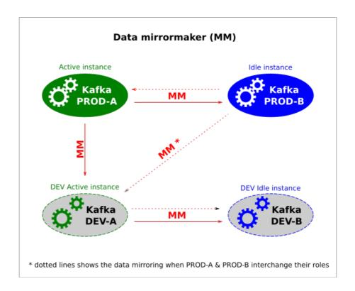
By having the same data on all Kafka environments we can safely apply blue-green setup and test changes in Kafka DEV under data load.
