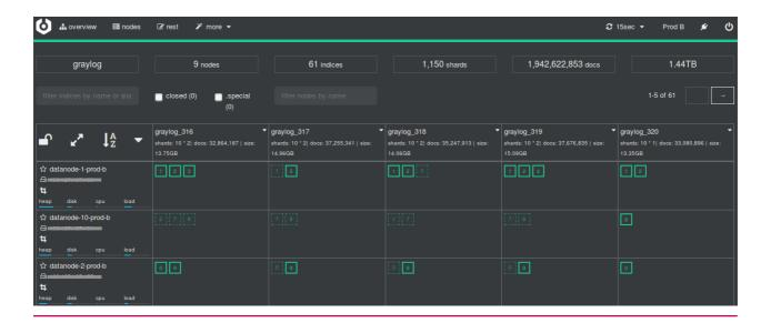
This way we quickly identified the problem of having most of the Shards allocated on a single node. Even after rotating the Active write Index we still had most of the Shards allocated to one specific node. We had to rotate Active write Index multiple times, since Graylog has a limit of reallocating maximum of two Shards in time by default when rotating the Index. Settings from Cerebro:
