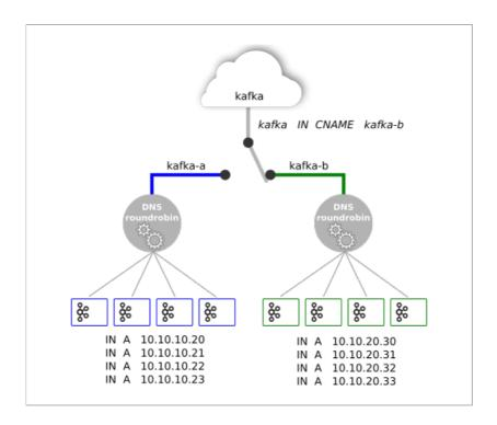
Within our data centres we use both options for various use cases. For Graylog we do blue-green switch for user access on HAProxy load balancers. For Apache Kafka we adopted DNS based switch since load balancing is managed by Kafka itself without need for dedicated LBs.
