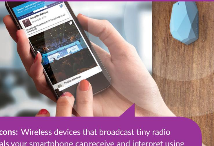
**Beacons:** Wireless devices that broadcast tiny radio signals your smartphone can receive and interpret using Bluetooth low energy (BLTE) technology.
