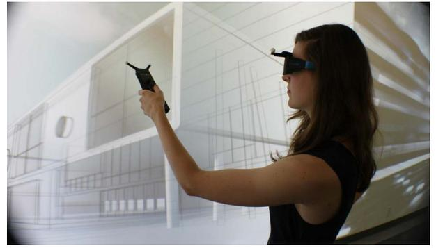
Our PPT wand is fully motion tracked and allows users to interact with 3D objects and navigate virtual worlds.
