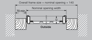
Fitting in the opening requires that the given dimensions be adhered to with greater accuracy.
