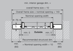
The recommended structural dimensions are recommended planning dimensions. Minimum sideroom, headroom and opening sizes are all based on these dimensions.
