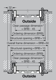
With an opening angle of less than 180°, the clear passage width is reduced.
