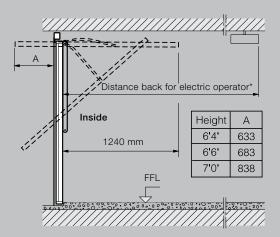
For doors with operator 40 mm headroom above top crossframe required.
