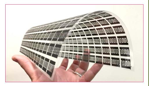
Screen Printing of Supercapacitor and Battery Electrodes
