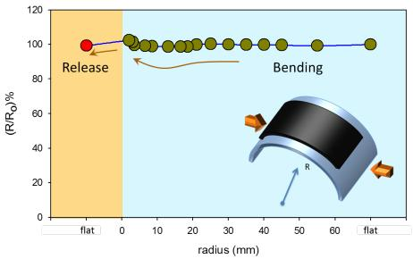
While there is a slight change in resistance under extreme bending (radius of curvature = 1.75 mm), the change is completely reversible when the sheet is returned to the flat state.
