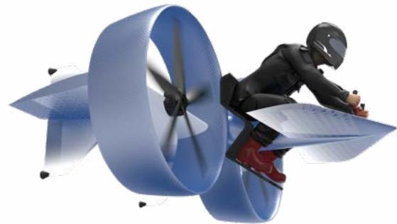
minimize noise while providing enough thrust for a controlled vertical take-off and landing and a top speed of over 100 km/h. Above all, safety is priority number one. The design has a low-power backup system and is capable of belly landing in case of emergency.
