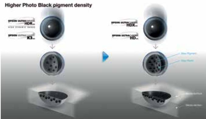
The proven Epson UltraChrome pigment inks offer smooth gradation and sharp definition, by utilising a three-level black ink technology that simultaneously employs black, light black and light light black ink to produce brilliant black density and grey balance. At the media surface, the UltraChrome HDX and HD matte and photo black inks achieve a much higher pigment density, ensuring the pigments do not penetrate too deeply when printing on third-party media.
