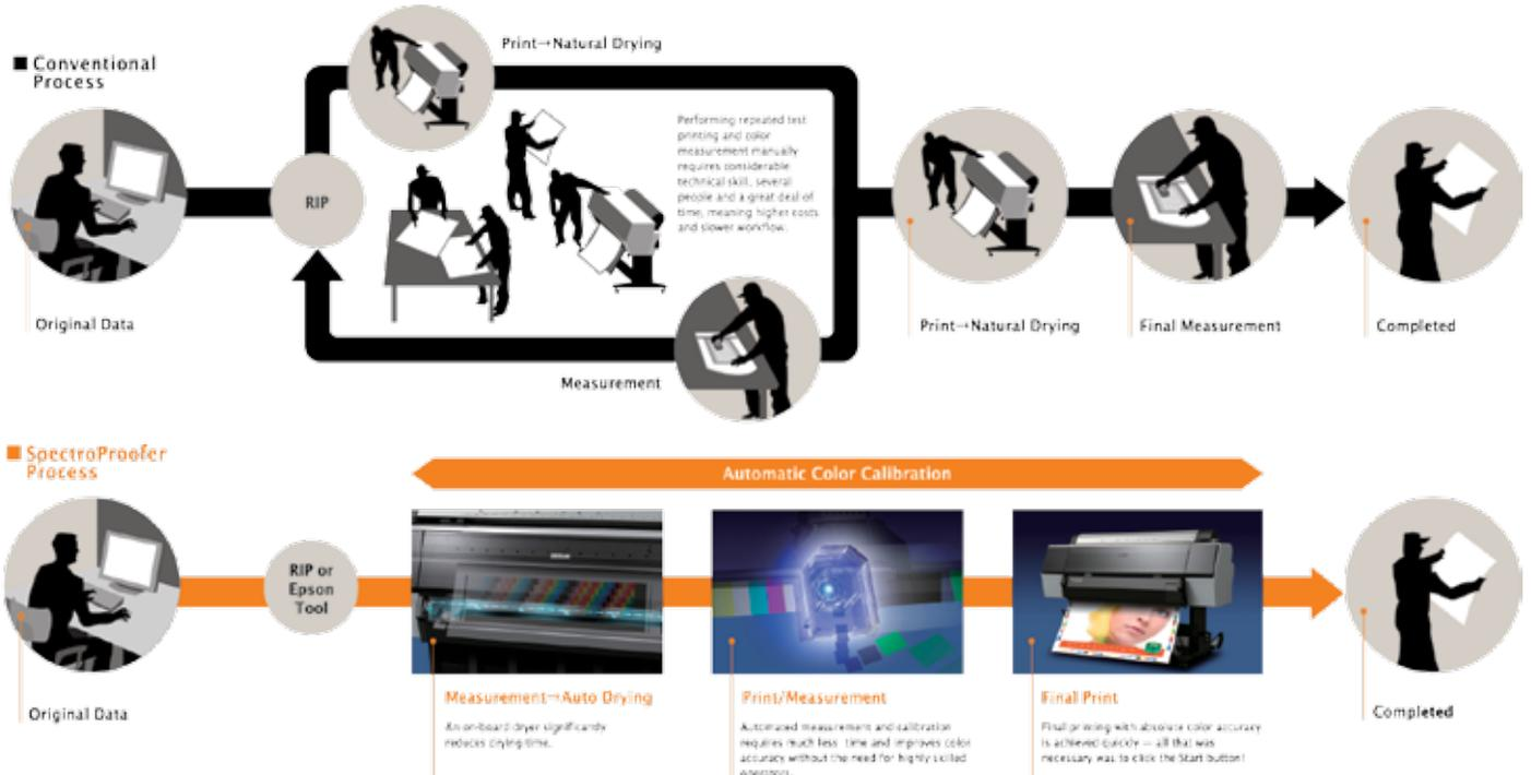
Available as an optional add-on, the ILS30 spectrophotometer (developed jointly with X-Rite) is essential to anyone who's looking for real efficiency in the proofing industry. It is capable of extreme measurement accuracy of below 0.2 dE-CMC. It simply attaches to the front of the printer, giving users the basis for an advanced colour management system.
