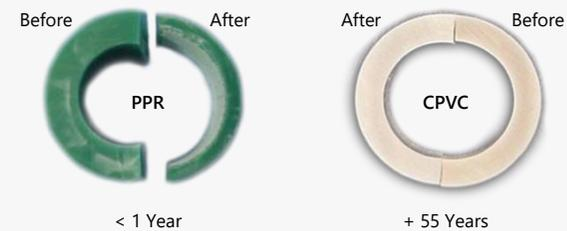
**FlowGuard® CPVC** and PPR pipes were tested to demonstrate the effects of chlorinated water. After running chlorinated water through a PPR pipe for 7,000 hours using a low water flow rate of ~0.1 gpm, the pipe wall was significantly eroded. Meanwhile, there is no notable erosion of a **FlowGuard® CPVC** pipe wall and no decrease in hydrostatic performance even after 55 years of use.
