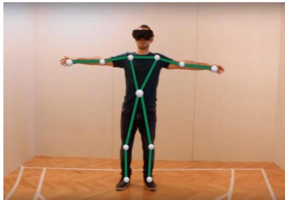
**Fig. 1.** The MRC is placed in front of the user to recognize the joints and place them inside the virtual environment.
