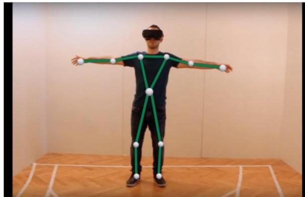
**Figure 1:** The MRC which is in front of the participant recognize the joints and place those inside the virtual world.
