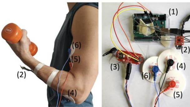
**Figure 2:** Hardware's placement on the user (a) – left: The placement over the participant. (b) – right: The Hardware used.
