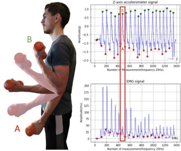
**Figure 1:** (a) – left: The bicep exercise demonstration, where Point A is the lowest point and Point B is the highest point. (b) – right: On the top is the Accelerometer signal, on the bottom is the EMG signal. The red rectangle demonstrates a full curl which corresponds to one full exercise curl.
