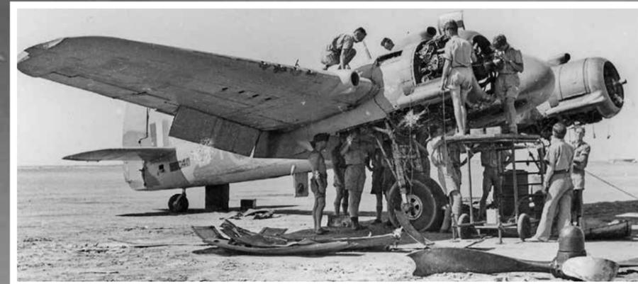
Left: T5040 undergoing repair after a forced landing judging by the bent propeller blades in the foreground. The Dark Green areas of the original Temperate Land Scheme appear to have been overpainted in either Light Earth or Mid Stone, leaving the serial number on a masked out rectangle of Dark Green.
