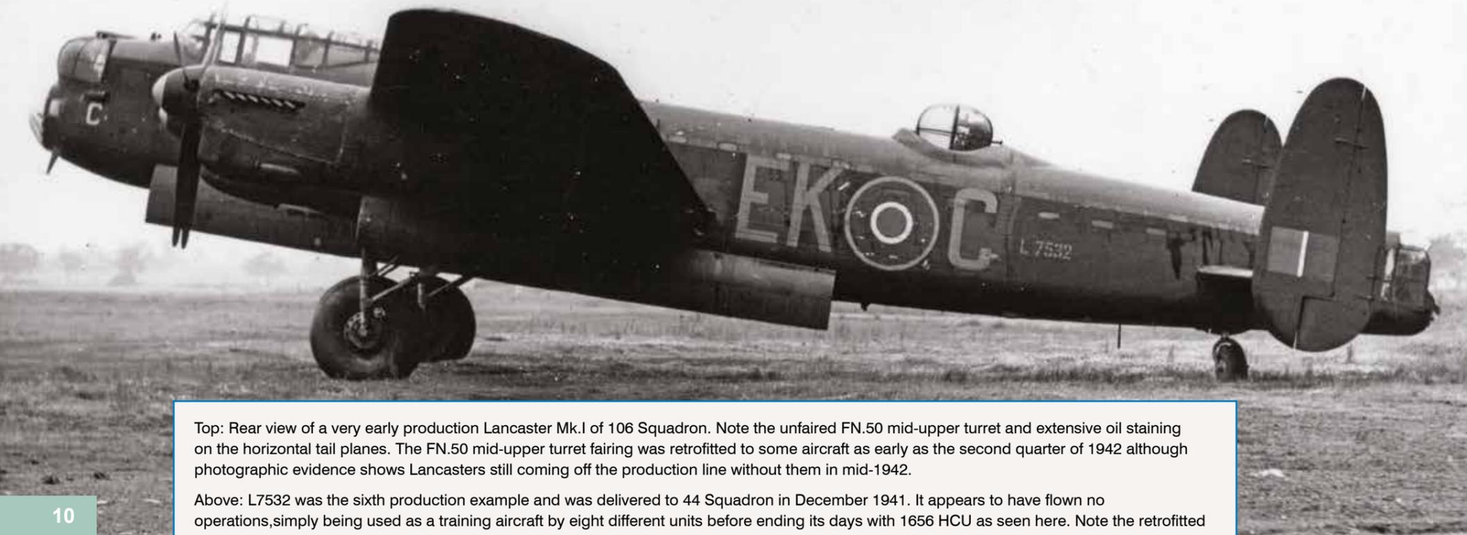
Top: Rear view of a very early production Lancaster Mk.I of 106 Squadron. Note the unfaired FN.50 mid-upper turret and extensive oil staining on the horizontal tail planes. The FN.50 mid-upper turret fairing was retrofitted to some aircraft as early as the second quarter of 1942 although photographic evidence shows Lancasters still coming off the production line without them in mid-1942.
