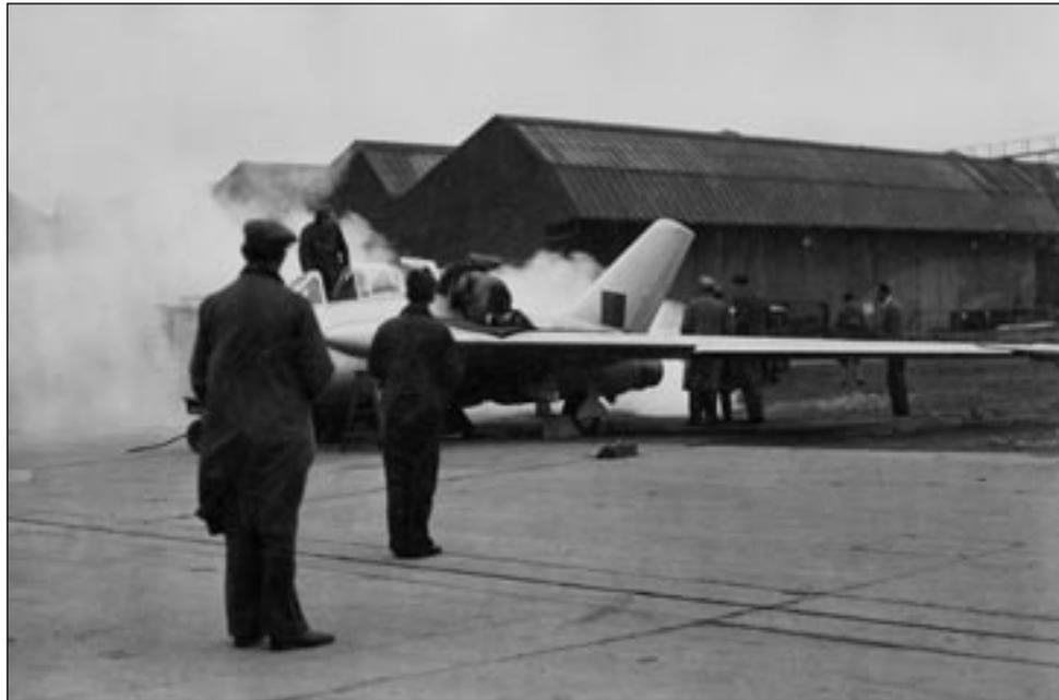
**A 'wet start' during an early engine run on TG/283. The clouds of paraffin vapour are from unburned fuel following a previous failed attempt to start. BAE SYSTEMS**
