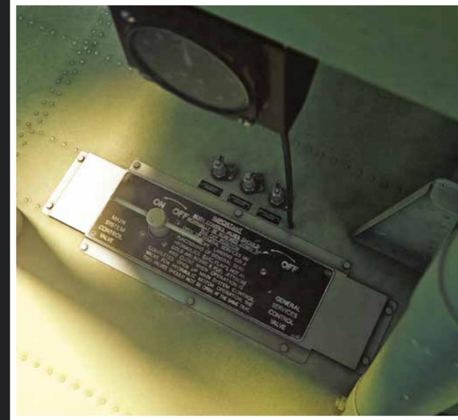
Contrary to what has been published before, the VSG motor was run off its own dedicated closed hydraulic circuit named as 'Main System'. The procedure during Operation Chastise was for the wireless operator to open the main system hydraulics about 10 minutes before the bomb run and turn the T-bar handle until the motor was spinning at 500rpm. Once the bomb was released, he would turn the T-bar handle the opposite way to stop the motor and then shut off the Main System hydraulics.
