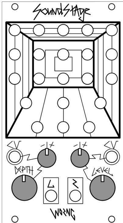
The SoundStage is the essence of a stereo mixer distilled into a powerful efficient package. It includes twenty-one inputs which pass through a combination of twenty resonant analogue filters for tonal control and mix down to a voltage controllable stereo output stage.
