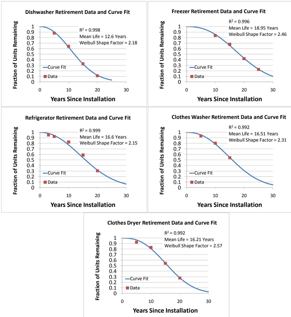
As seen in Figure 3, the Weibull distribution appears to be a good choice curve-fitting to appliance retirement data. The data were then normalized by mean lifetime to illustrate the similarity in the *shape factor* of the mortality curves across these appliances. Figure 4 shows that appliance mortality behaves in a very consistent manner across multiple residential appliances, when normalized by mean lifetime.
