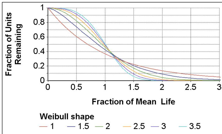
Data for each appliance was fit with a Weibull distribution, adjusting the scale and shape factors using least-squares regression. The regression results are summarized below in Table 2.
