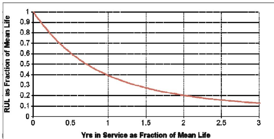
Using Figure 6, one can see for instance that if a product has an EUL of 10 years and has been in service for 10 years, one could expect the product to last for an additional 3.9 years (or  $0.39 \times 10$  years, where 0.39 is the y-axis value read at the x-axis value of  $10/10 = 1$ ). Likewise, if the product were in service for 20 years (or  $2 \times$  EUL), one could expect the product to last an additional 2 years (or  $0.2 \times$  EUL), on average.
