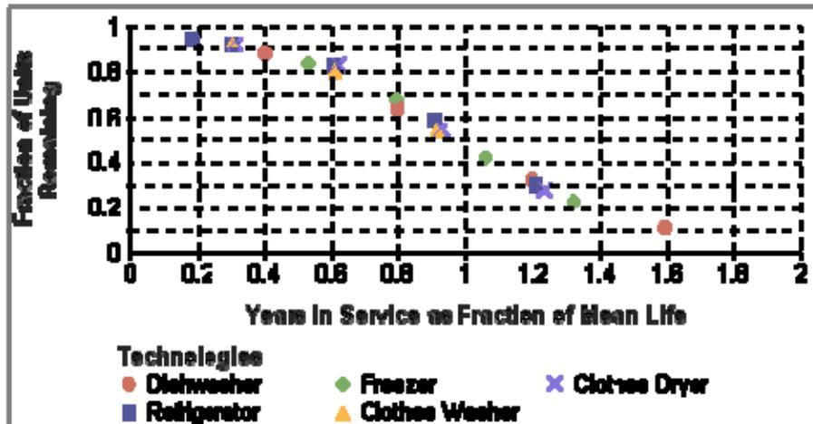
When the normalized appliance mortality data are fit to a Weibull distribution, the outcome is a tightly constrained range of shape factors across appliance types. Figure 5 shows the tight range of Weibull curves fit to the normalized data.
