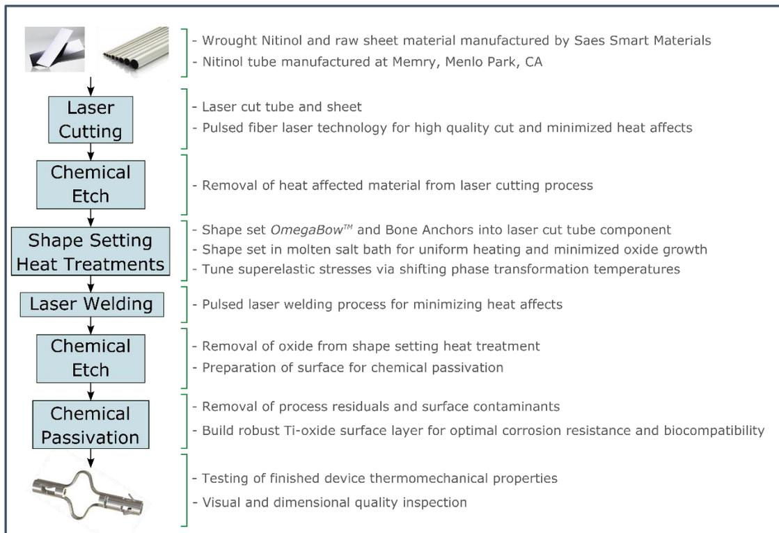
Figure 3: Memry's manufacturing process flow.
