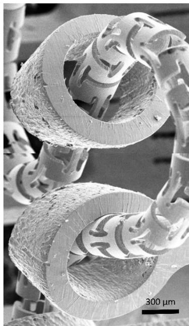
*Figure 2: Laser cutting process extremes. Fiber cut tube (5 mm OD x 0.56 mm wall) vs. Femto cut tube (0.343 mm OD x 0.044 mm wall). Stents shown are in as-cut condition where a typical re-cast surface structure is observed on the component cut using the thermal based fiber laser cutting process.*
