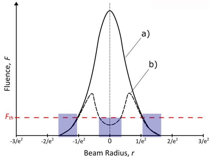
Figure 4: Laser fluence of a Gaussian laser beam expressed in 2D.  $F_{th}$  represents the threshold fluence for the ablation of Nitinol. Below this threshold the laser energy will be transmitted into the bulk material through thermal conduction. Curve a) illustrates typical undistorted beam having fluence below  $F_{th}$  only at tails. Curve b) illustrates a distorted beam profile where the fluence drops below  $F_{th}$  at the center.
