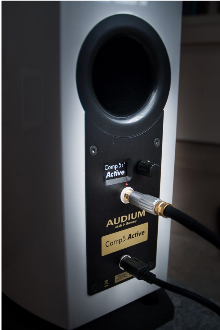
AUDIUM Comp 5.2 Active - the connection terminal with user interface (Photo: Falk Visarius)
