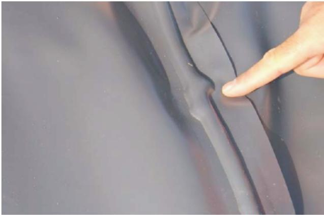
**Figure 6. Aneurysm in 0.75 mm PVC geomembrane seam**
