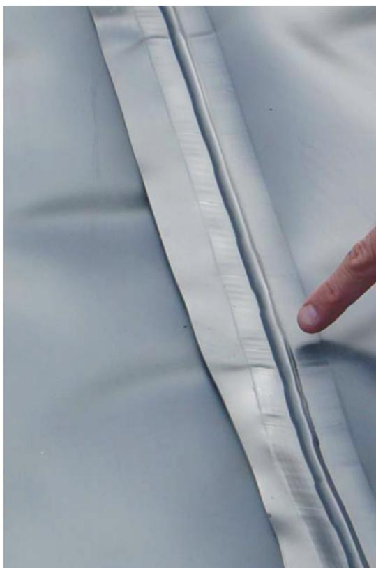
Figure 1. Air channel test performed in 0.75 mm PVC geomembrane seam
