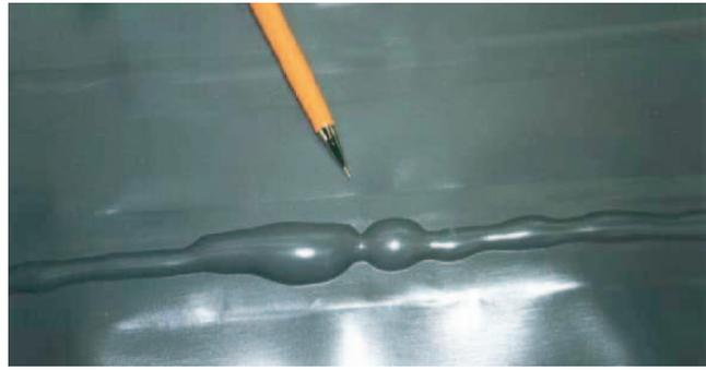
**Figure 10. Inflated air channel in 0.75 mm-thick geomembrane at room temperature (22.8°C) with a problematic seam (photo courtesy of Fred Rohe, Environmental Protection, Inc.)**
