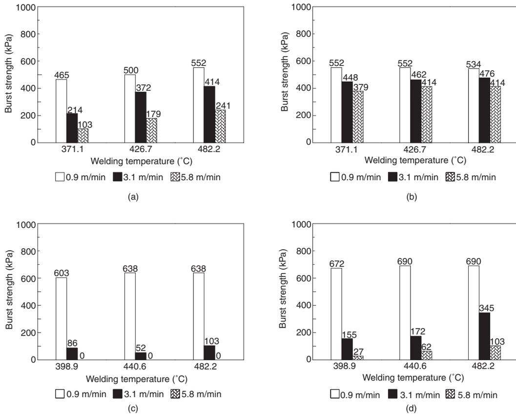
Figure 7. Seam burst pressures for 36 hot wedge welded seams, burst at 35.0°C: (a) 0.75 mm, sheet temperature 10°C; (b) 0.75 mm, sheet temperature 32.2°C; (c) 1.00 mm, sheet temperature 15.6°C; (d) 1.00 mm, sheet temperature 37.8°C
