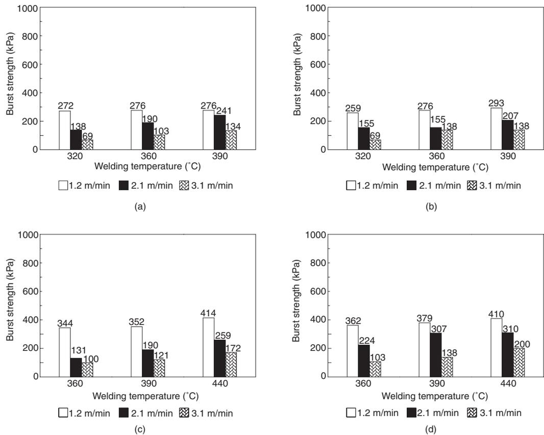
Figure 5. Seam burst pressures for 36 hot air welded seams, burst at 46.7°C: (a) 0.75 mm, sheet temperature 10°C; (b) 0.75 mm, sheet temperature 26.7°C; (c) 1.00 mm, sheet temperature 15.6°C; (d) 1.00 mm, sheet temperature 32.2°C
