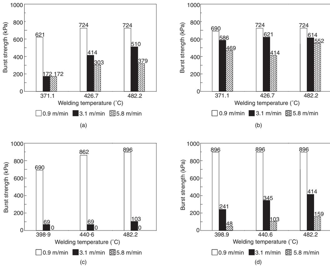
Figure 6. Seam burst pressures for 36 hot wedge welded seams, burst at 22.8°C: (a) 0.75 mm, sheet temperature 10°C; (b) 0.75 mm, sheet temperature 32.2°C; (c) 1.00 mm, sheet temperature 15.6°C; (d) 1.00 mm, sheet temperature 37.8°C
