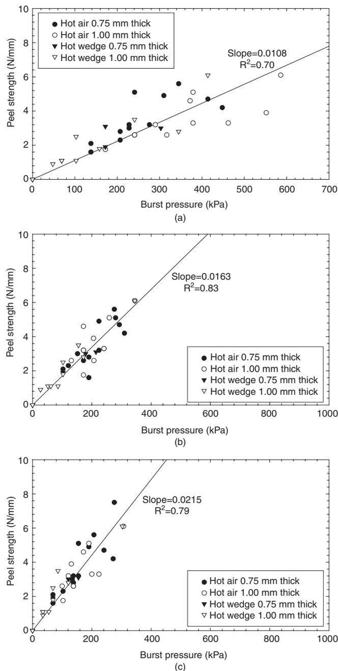
Figure 12. Relationship between burst pressure and peel strength for all non-FTB seams and 0.75 mm and 1.00 mm-thick geomembrane and hot air and hot wedge welding: (a) 22.8°C; (b) 35.0°C; (c) 46.7°C
