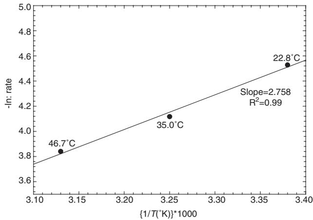
**Figure 14. Arrhenius relationship between the ratio of peel strength and burst pressure to sheet temperature**
