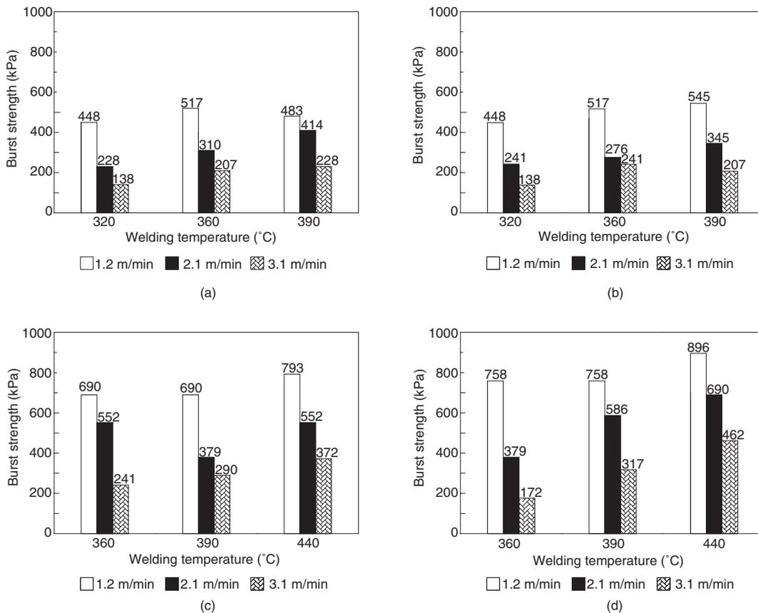
Figure 3. Seam burst pressures for 36 hot air welded seams, burst at 22.8°C: (a) 0.75 mm, sheet temperature 10°C; (b) 0.75 mm, sheet temperature 26.7°C; (c) 1.00 mm, sheet temperature 15.6°C; (d) 1.00 mm, sheet temperature 32.2°C
