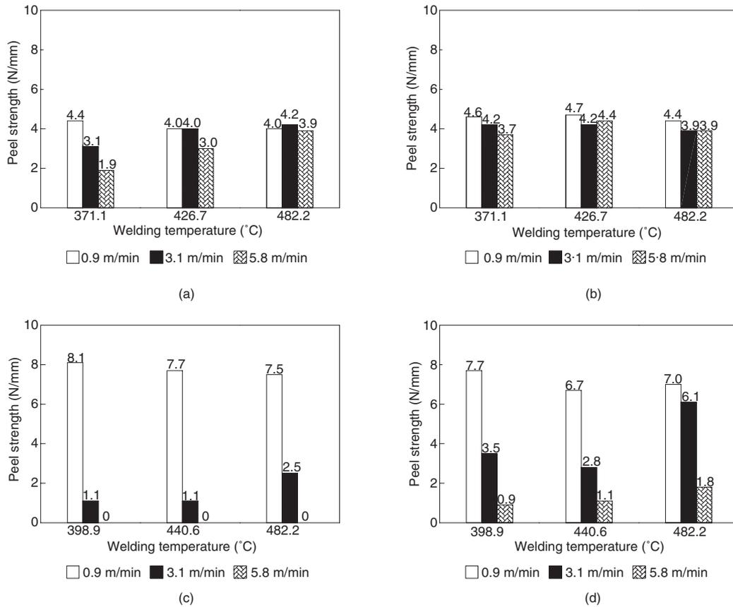
**Figure 2.** Seam peel strengths for 36 hot wedge welded seams: (a) 0.75 mm, sheet temperature 10°C; (b) 0.75 mm, sheet temperature 32.2°C; (c) 1.00 mm, sheet temperature 15.6°C; (d) 1.00 mm, sheet temperature 37.8°C
