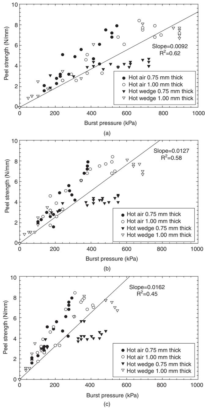
Figure 11. Relationship between burst pressure and peel strength for hot air welded seam. Sheet temperature: (a) 22.8°C; (b) 35.0°C; (c) 46.7°C
