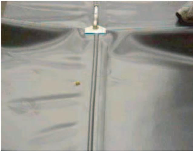
**Figure 9. Inflated air channel in 0.75 mm-thick geomembrane in the field (photo courtesy of Fred Rohe, Environmental Protection, Inc.)**
