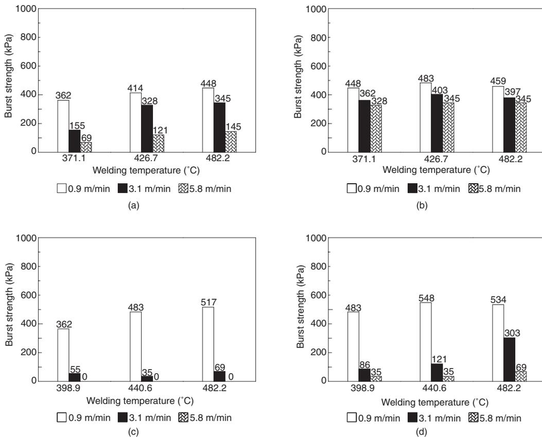
Figure 8. Seam burst pressures for 36 hot wedge welded seams, burst at 46.7°C: (a) 0.75 mm, sheet temperature 10°C; (b) 0.75 mm, sheet temperature 32.2°C; (c) 1.00 mm, sheet temperature 15.6°C; (d) 1.00 mm, sheet temperature 37.8°C
