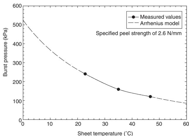
**Figure 13. Burst pressure required to verify a specified peel strength of 2.6 N/mm at various sheet temperatures**
