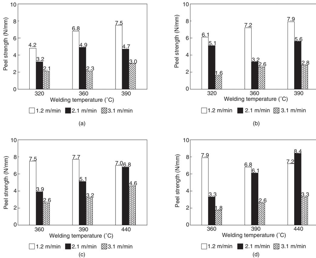
Figure 1. Seam peel strengths for 36 hot air welded seams: (a) 0.75 mm, sheet temperature 10°C; (b) 0.75 mm, sheet temperature 26.7°C; (c) 1.00 mm, sheet temperature 15.6°C; (d) 1.00 mm, sheet temperature 32.2°C
