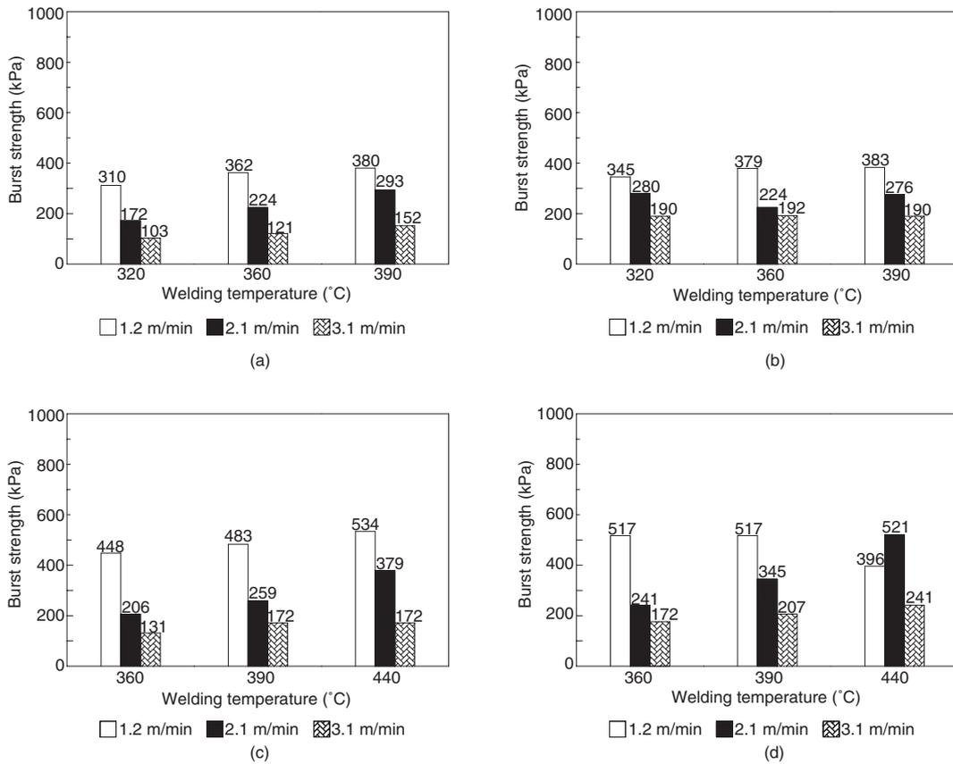
Figure 4. Seam burst pressures for 36 hot air welded seams, burst at 35.0°C: (a) 0.75 mm, sheet temperature 10°C; (b) 0.75 mm, sheet temperature 26.7°C; (c) 1.00 mm, sheet temperature 15.6°C; (d) 1.00 mm, sheet temperature 32.2°C
