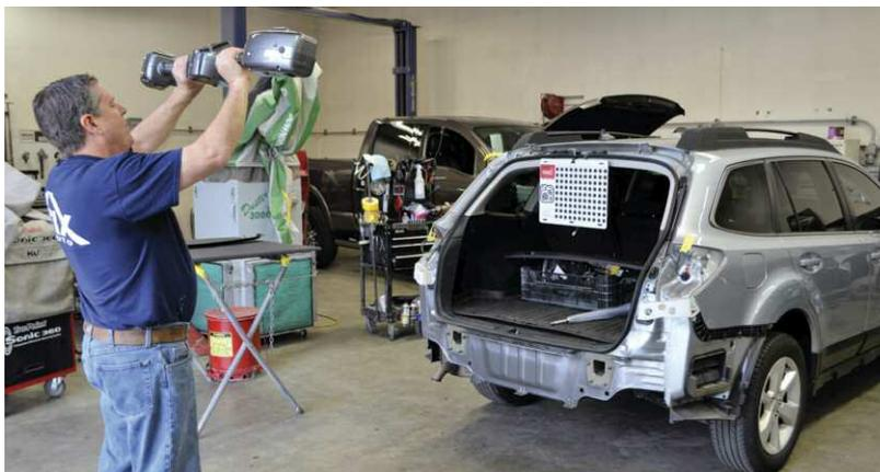
The *Matrix Wand* allows employees at *Fix Auto Puyallup* to get a more accurate picture of the repairs needed.
