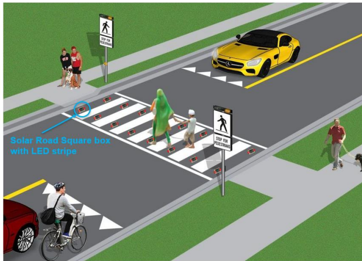
■ Solar Road Square box ● Embedded LED stripe on Solar Road Square box
