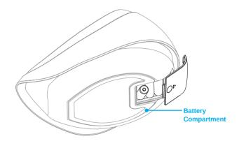
Insert 3 AA batteries into the batteries compartment located at the underside of the Smartbowl.
