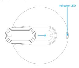
Before its first usage, charge the SmartTag to activate its wireless connectivity by inserting it into the charging slot.
