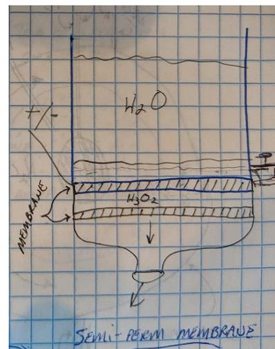
*Rough sketch of "Semi-permeable membrane" (carbon) method of filtration*
