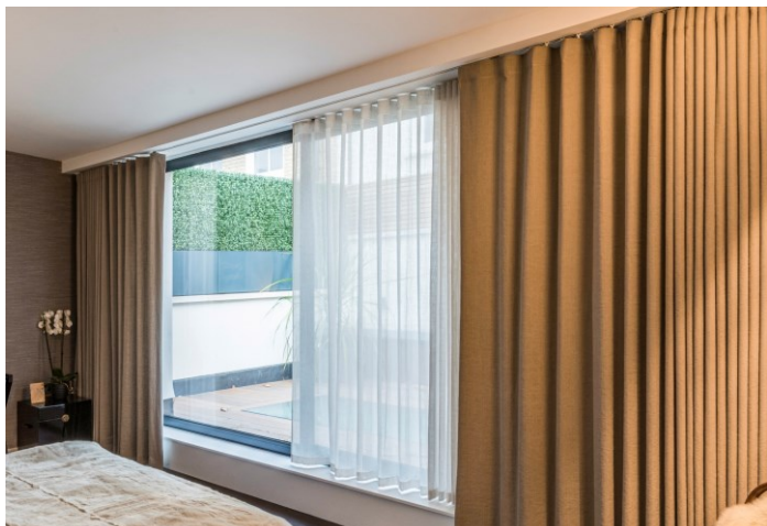
Dual RT1F with SG51MB1F and SG51RB1F, tracks with 180mm spacing.
