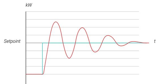
While ideally SCADA software and equipment will be selected and configured to reduce the data latency, the controller can be fine-tuned to contend with feedback-lag without losing control.
