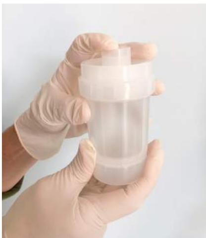
**FIGURE 4.17** ELUTOR SNAPPED ONTO THE FILTER
