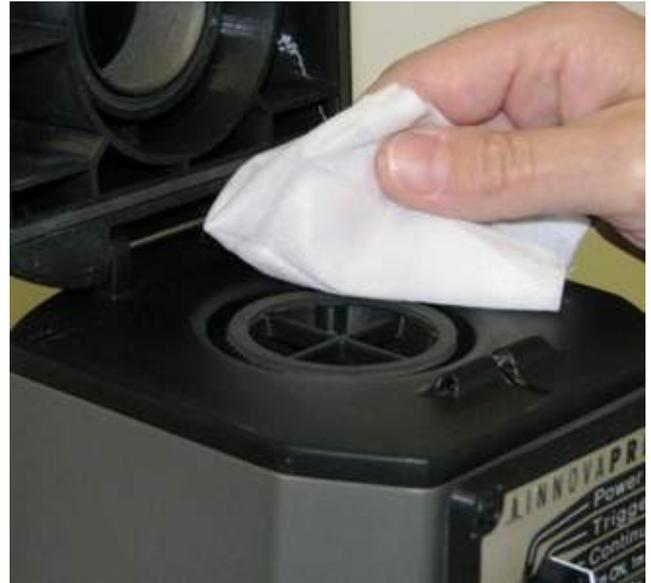
**FIGURE 4.21** CLEANING INTERIOR SURFACES
