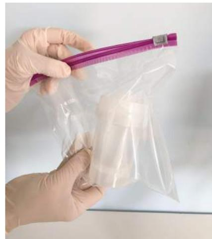
**FIGURE 4.18** ASSEMBLY IS BAGGED AND READY FOR TRANSPORT TO THE LABORATORY
