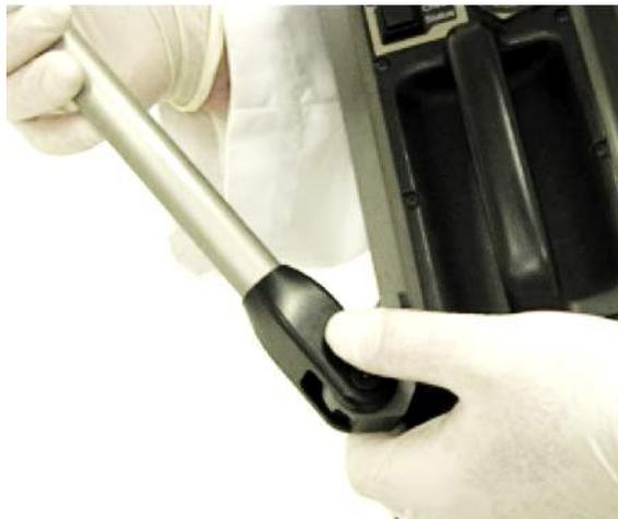
**FIGURE 4.2** UNLOCKING AND UNFOLDING LEG
