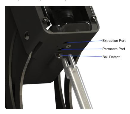
**FIGURE 4.6 TIP INTERFACE PORT DETAIL**
