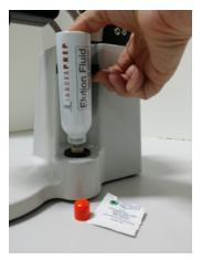
FIGURE 4.5 INSTALLING AND REMOVING FLUID CANISTERS
