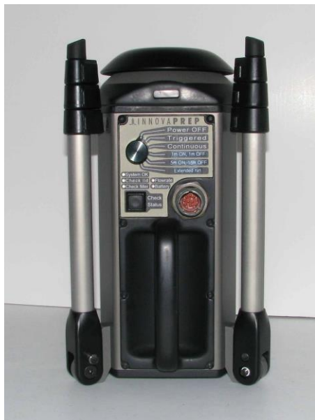
Figure 2-8. Dry Filter Collector
