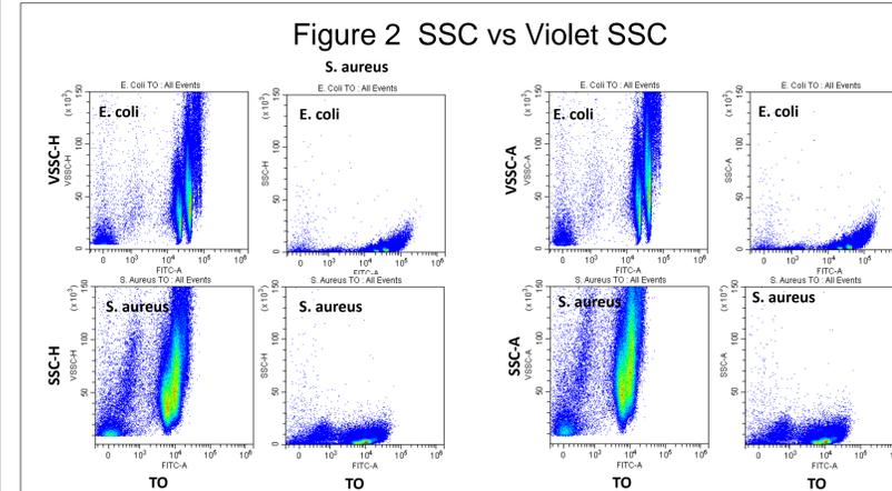
Figure 2 SSC vs Violet SSC. CytoFLEX instruments configured with Violet Side Scatter (VSSC) has better resolution for E. coli and S. aureus compared to the standard Side Scatter (SSC) from the 488nm laser.
