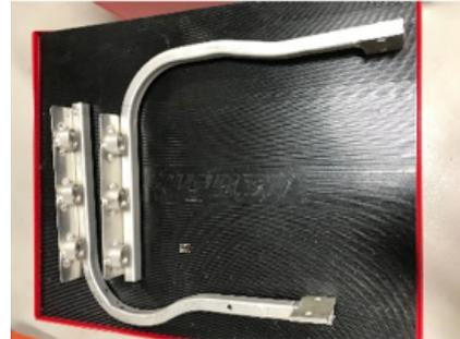
Rayburn's 2nd version of the customized bracket that move with the wheel when the wheel is turning.
