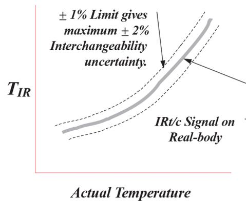
5. An IRT/c's full performance *cannot be accurately checked with a black-body*. Standard laboratory black-bodies can be used for pass-fail or reproducibility testing only. Contact Exergen for availability of specialized test devices.
