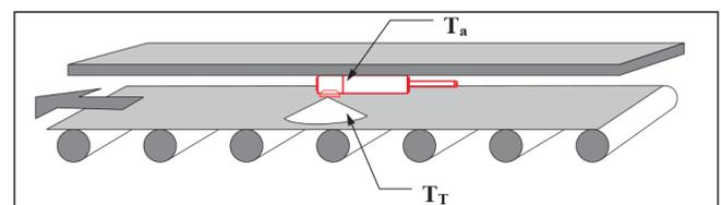
A second effect on linear range is the effect of target surface temperature on ambient temperature, and therefore the reflected component of radiation to the sensor. As target temperature increases within a process, the increased radiation heat transfer to the surroundings will cause the target ambient radiant background to also increase in temperature.
