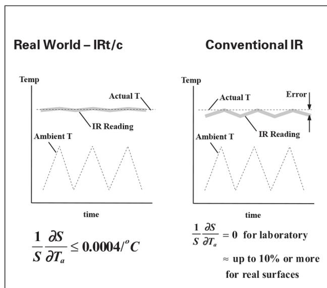
temperature. This equation describes the output of the IRt/c, including a gray-body assumption of emissivity = 0.9, and that the sensor itself is at the same temperature as the environment.
