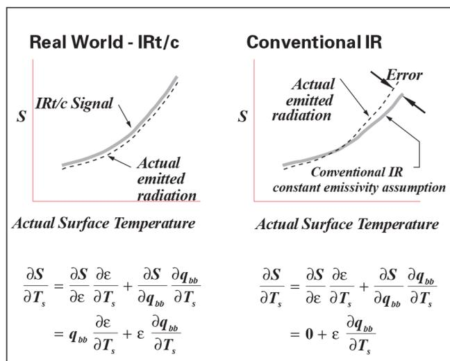
Note that the conventional IR device loses one term of the signal change with respect to surface temperature. When the IR signal is converted to a temperature indication, the signal in the conventional device is linearized, whereas in the IRT/c the signal is unchanged.
