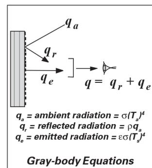
Accordingly, for a black-body  $\epsilon = 1$ , and therefore  $\rho = 0$ . But for a gray-body  $\epsilon < 1$  and therefore  $\rho > 0$ , and the reflected radiation due to ambient temperature must be considered. Refer to Tech Note No.
