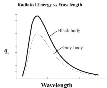
An important element which is missing when working with black-bodies, but present with graybodies is reflected radiation.
