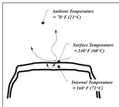
The IRt/c Heat Balance Series Infrared Thermocouples actually calculate the internal temperature by solving the equation that describes the heat balance between internal, surface, and ambient temperatures, and produce an *unpowered thermocouple signal that represents the internal temperature!*
